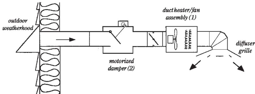
TYPICAL MAKE-UP AIR SYSTEM: DUCT HEATER/FAN ASSEMBLY
