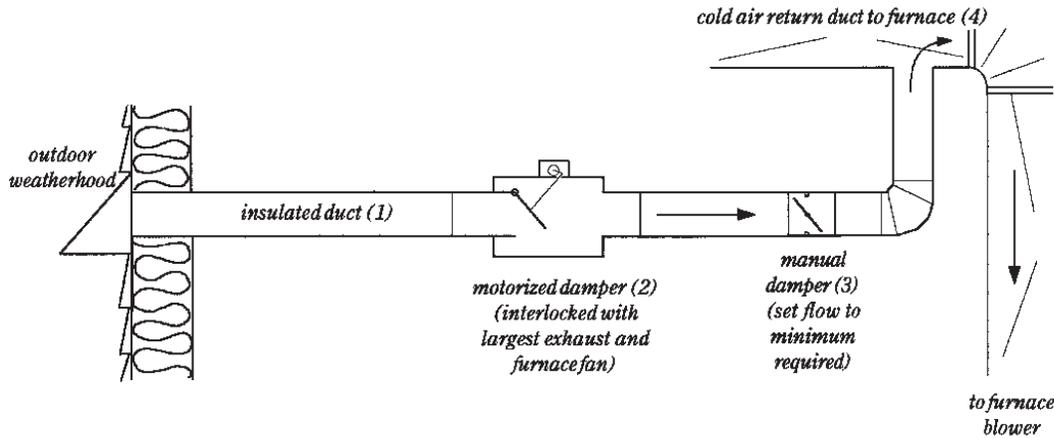
TYPICAL MAKE-UP AIR SYSTEM: FORCED AIR HEATING SYSTEM
